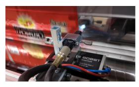
**Registron® register control system** Exceptionally accurate and rapid print-to-print register control. Corrections are quickly and precisely done while machine downtime and waste are reduced to a minimum.
